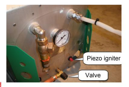
or hands over/under the device when igniting. It may ignite with a "BOOF" and the flames can shoot out of the device for a short second. The flames can be seen and controlled through the hole in the side panel of the device.
